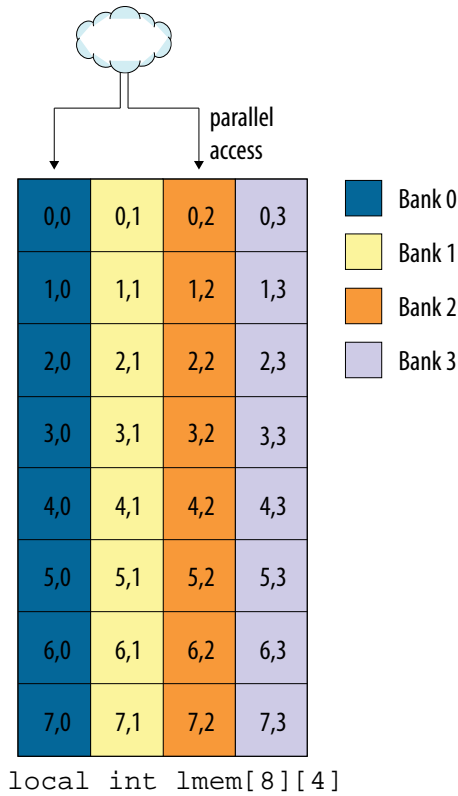
Figure 84. Parallel Access to an 8 x 4 Local Memory System with Four 4-Byte-Wide Memory Banks
